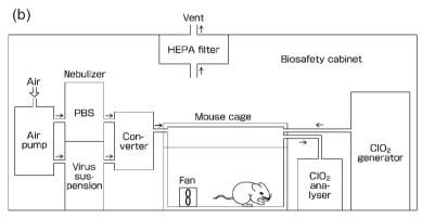
**Fig. 1.** (a) Schematic structure of a CIO<sub>2</sub> generator. (b) Experimental set-up for exposure of mice to influenza A virus aerosols and CIO<sub>2</sub> gas.
